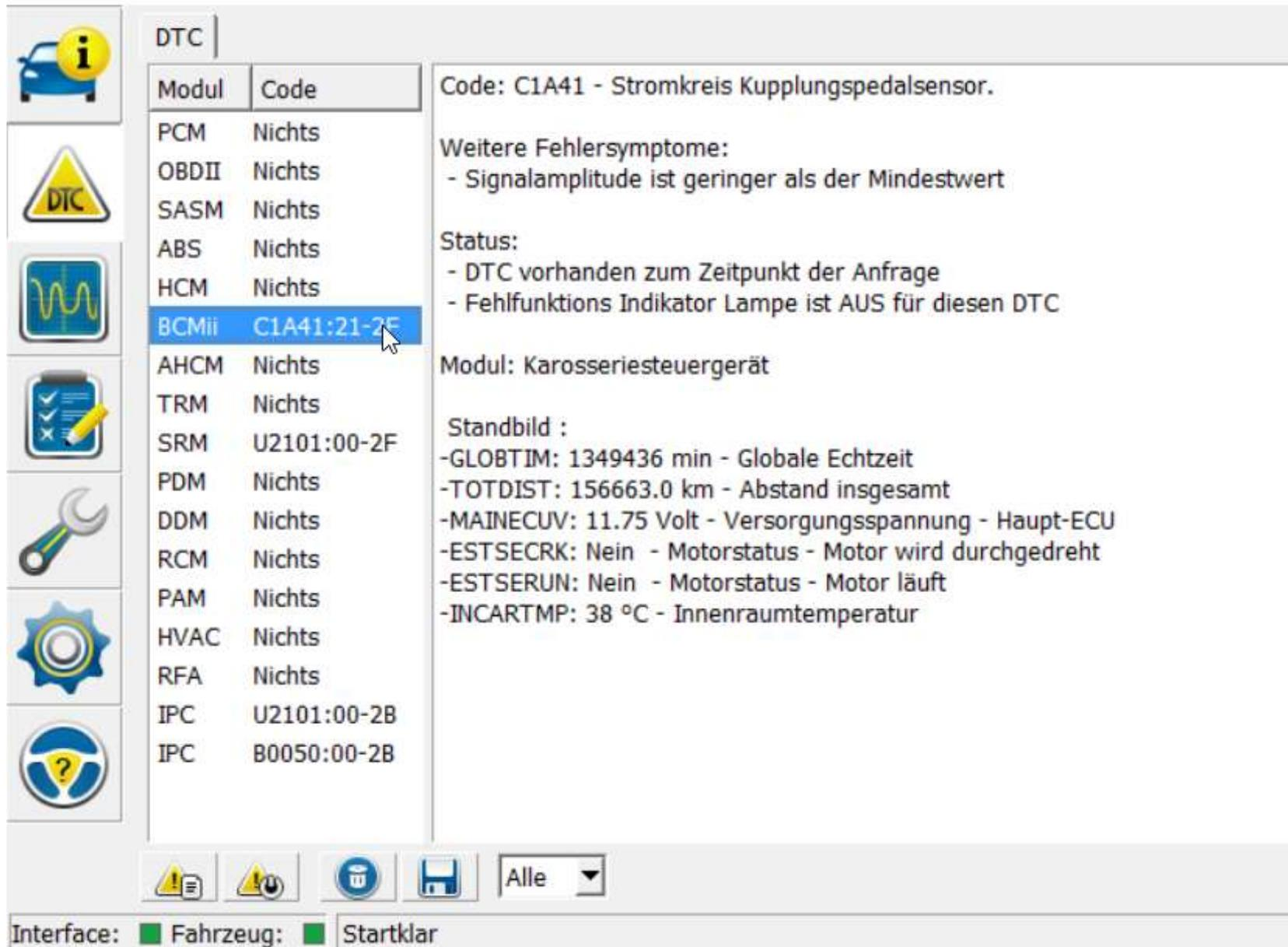
The image shows the FORScan diagnostic software interface. On the left is a vertical toolbar with icons for information, DTC, waveform, clipboard, wrench, gear, and steering wheel. The main area is titled 'DTC' and contains a table of diagnostic trouble codes. The code 'C1A41:21-2F' is selected, and its details are shown on the right. The status indicates the DTC is present and the indicator lamp is off. The 'Standbild' (snapshot) section provides various vehicle parameters.
